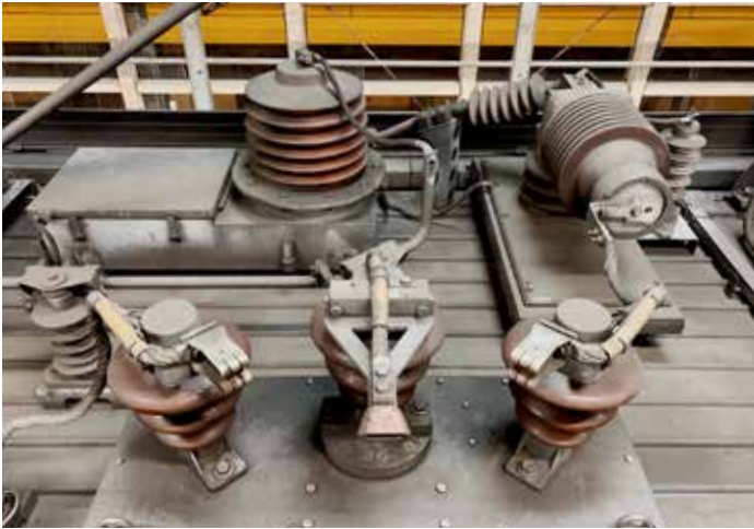
Current system selection relay on the roof of the TramTrain.
